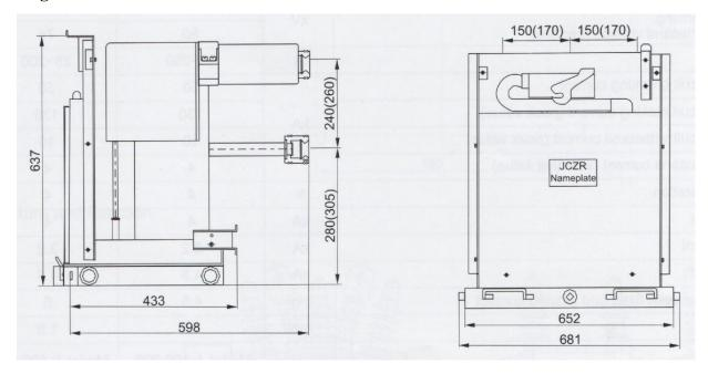
7.2kv dimensions (the dimensions in brackets is for 12kv)
